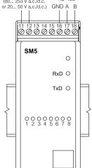
Fig 2. Electrical connections of SM5 logic input module
