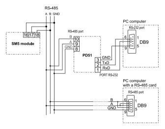
Fig. 3 Way of the RS-485 interface connection.
